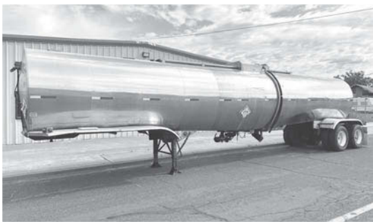
1988 BARBEL STAINLESS STEEL TANK TRAILER , 7000 GALLONS, 1 COMPARTMENT, DOUBLE CONICAL / CENTER DISCHARGE, SPRING RIDE SUSPENSION, 295/75R22.5 TIRES, STEEL WHEELS, 3" STAINLESS QRB STYLE VALVE AT THE CENTER, HOSE TRAY RIGHT SIDE, 60% BRAKES, 60% TIRES, BAR-BEL 42' 7000 GAL SS TANKER
