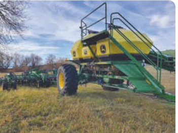
2015 John Deere 1910 cart with a 2015 John Deere 35' 1830 drill. 7.5" spacing, 3 tank cart, front tank is 150 bu., rear tank is 200 bu. and center tank is 750 gal. Liquid starter tank on 3 sections
