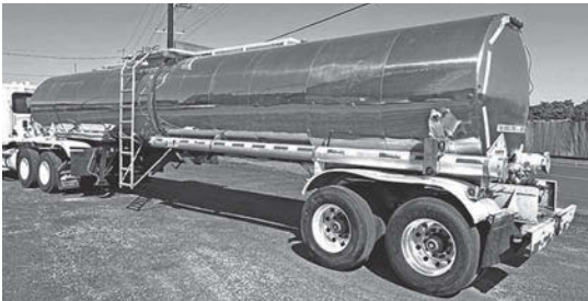
1985 FRUEHAUF STAINLESS STEEL TANKER , 6700 GALLONS, STRAIGHT ROUND / REAR DISCHARGE, 3" QRB STYLE SS VALVE, AIR RIDE SUSPENSION, 295/75R22.5 RUBBER, ALL ALUMINUM WHEELS, HOSE TUBES EACH SIDE, 80% RUBBER, 70% BRAKES.....
