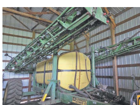
SUMMERS ULTIMATE NT SUSPENDED BOOM SPRAYER, 90' Booms, 1500 Gal Poly Tank, 7 Section Control, Boom Height, Mix Tank... $11,000
