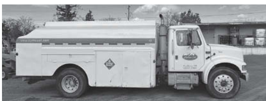
1995 INTERNATIONAL 4900, DOUBLE PUMPER, DT 466, 250 HP, 6 PLUS 1 TRANS, 11R22.5 RUBBER 70%, SPRING SUSPENSION, 2500 gal Progress STEEL 4 COMPARTMENT TANK, 800 / 700 / 500 / 500, 2 PUMPS AND DELIVER SYSTEMS, NON PRINTED TICKET METER HEADS, DRY BRAKES AND SWING HOSES BETWEEN THE COMPARTMENTS, BARREL BOOT, REAR PINTLE WITH AIR AND ELECTRICAL PLUS A RECEIVER HITCH. GREAT CONSTRUCTION FUELER OR FARM FUELER. 14,906 miles
