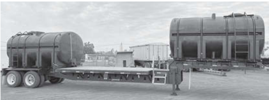
2024 DEMCO LIQUID TENDER, 42' LONG, 3250-GAL FRONT AND REAR TANKS, AIR AND ELECTRICAL TO BOTH TANKS, 24" PIN SETTING, STEEL WHEELS, 295 75R 22.5 LOW PRO TIRES, SPRING SUSPENSION, BLACK CORROL "ANTI CORROSION PAINT", ALUMINUM APPROACH STEPS EACH SIDE, COMING IN EARLY OCTOBER LET'S KILL SOME WEEDS!
