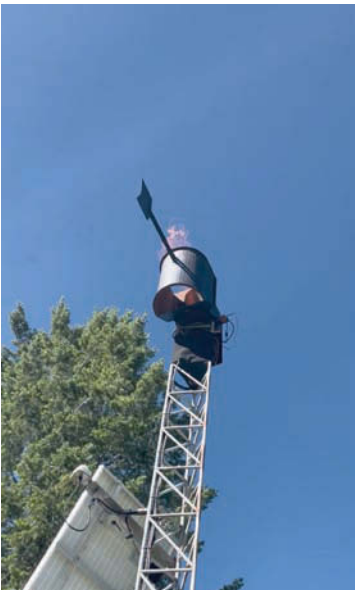
Courtesy Idaho Power Ground generation equipment used for cloud seeding.
