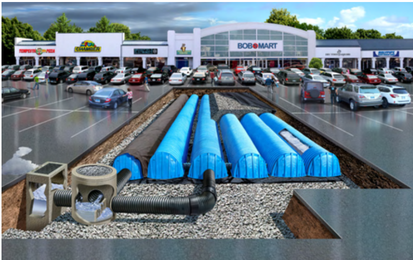
Figure K : Underground detention basins Source: Cultect, Inc, 2024
