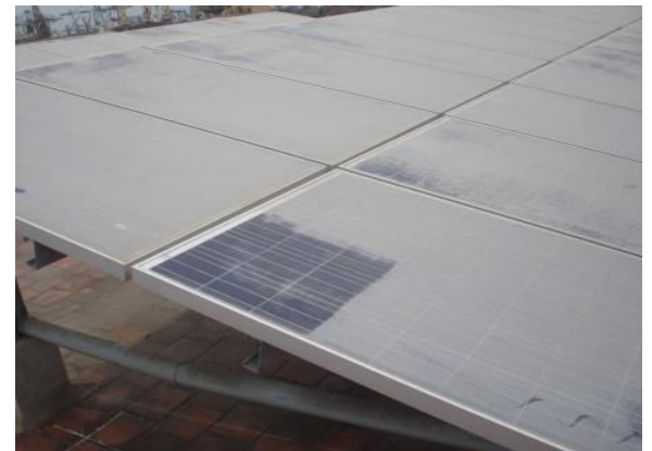
Left top corner coated with "Solar Glass Shield and the difference after 21 days
