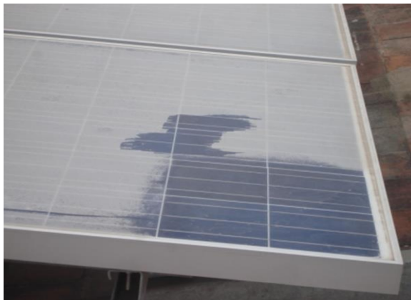
Left bottom corner of the panel coated with "Solar Glass Shield" and the difference after 21 days.
