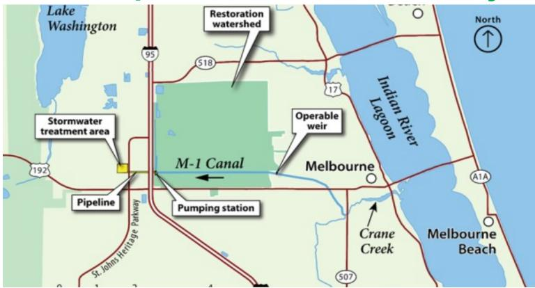
The St. Johns River Water Management District will soon begin the Crane Creek/M-1 Canal Flow Restoration Project Restoration Project, designed to reduce stormwater runoff flowing to the Indian River Lagoon.
