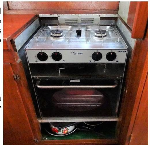
I fitted a vent at the back to act as a reflector. (Seen in the pic below) This is a standard vent available from any chandlery, bent to fit.
