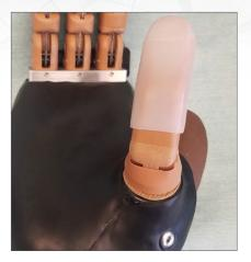
12. Install thumb tip with supplied phillips head screw and lock nut
