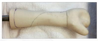
Duplicate model with silicone interface and use new plaster model for lamination to preserve silicone interface
