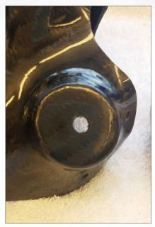
Remove M-Thumb dummy and Drill 3/16 hole in center.
