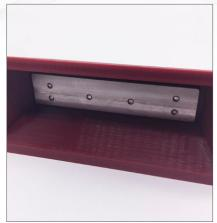
13. Place M-finger mount bracket on the inside of lamination. Mark holes, remove bracket and drill out with 1/8 inch bit
