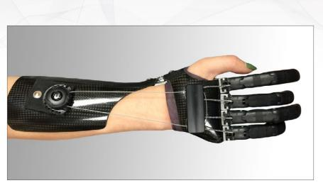
16. Install BOA cable connector or preferred cable attachment method in proper location as shown above. BOA should set while patient goes through range of motion to insure optimal location.
