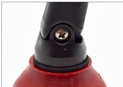
Disassemble M-Thumb by removing the Phillips screw on the side.
