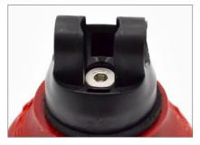
Install thumb base and screw through center hole. Tighten with 3/32" Allen wrench.
