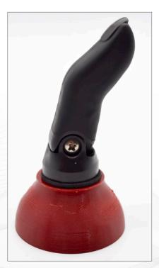
Install thumb assembly on base. Tighten Phillips screw to lock in place.
