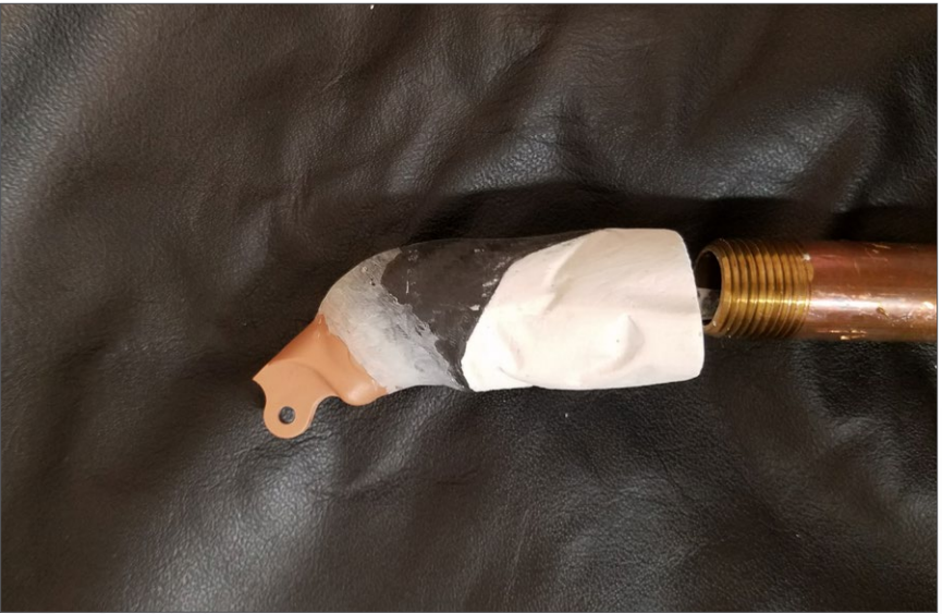
31. Prep for plaster pour and last layer of prepreg
