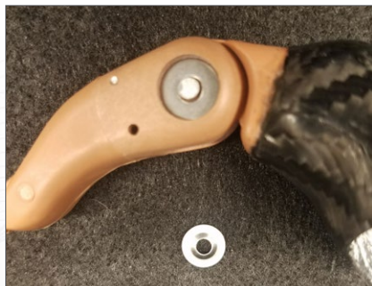
36. Insert pin. Place flat washer 1st, then place beveled washer above. Using light even pressure, push beveled washer down. If you push washer too far down, finger won't spring back up properly.
