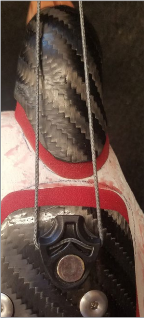
38. Attach PMF anchor and pull up to finger base slot and out the tip
