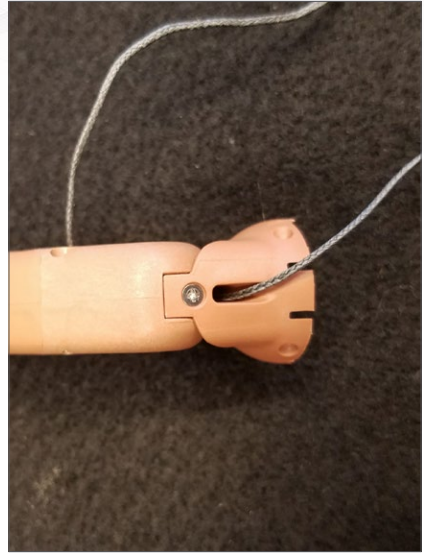
26. String gray PMF cord through m-finger base up to the right side of finger
