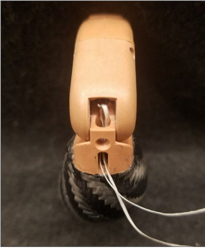
37. Restrung to pull spring down and screw onto base
