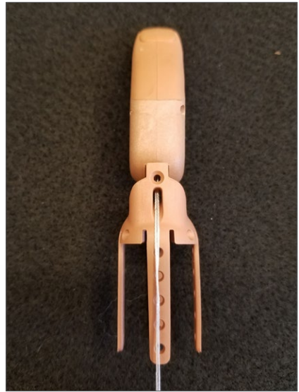
23. Thread string through spring hole and pull finger tip to the base
