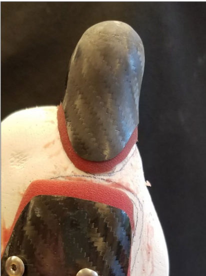
27. Scuff prepreg socket for adhesion of 60 sec epoxy and align finger to patient
