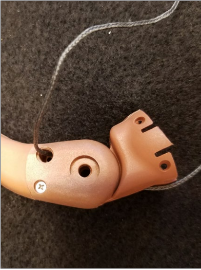
26. String gray PMF cord through m-finger base up to the right side of finger
