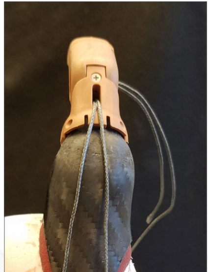
27. Scuff prepreg socket for adhesion of 60 sec epoxy and align finger to patient
