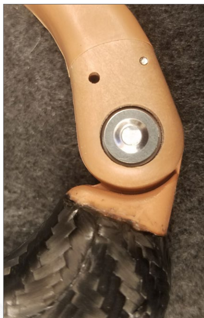
36. Insert pin. Place flat washer 1st, then place beveled washer above. Using light even pressure, push beveled washer down. If you push washer too far down, finger won't spring back up properly.
