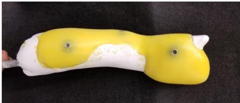
2. Duplicate model of silicone interface and use new plaster model for lamination to preserve silicone interface
