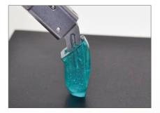
Press fingertip onto finger and hold in place until glue sets. Use rubber padding to prevent slipping.
