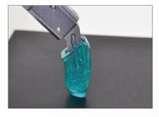
Press fingertip onto finger and hold in place until glue sets. Use rubber padding to prevent slipping.
