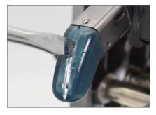
Wedge a flat-edge screw driver into the slot created and pry tip off finger tip.
