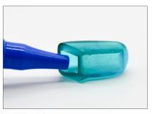
Apply a small amount of super glue on either side of the inner surface of the tip
