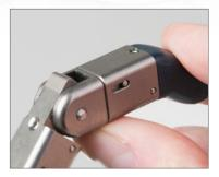
Apply pressure to the back of the thumb tip, which causes the thumb tip to ratchet into flexion. Once the desired position is determined, pressure can be removed from the thumb tip and the tip would be locked in to position.
