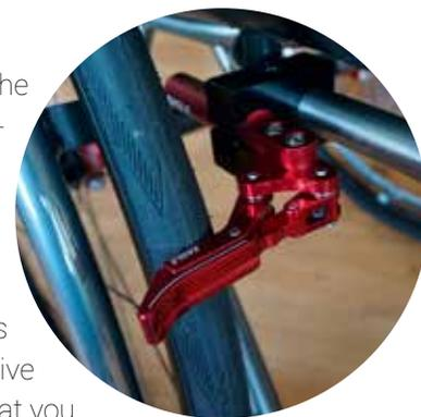
Remember that the brakes are intended as parking brakes, not as service brakes. If you use the parking brakes while you are in motion, there is a risk that you will lose control of the direction of the wheelchair and it may stop very suddenly, which may cause you to collide with something or roll out of the wheelchair.
