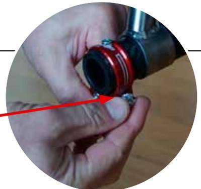
*Tightening the clamp screw*
