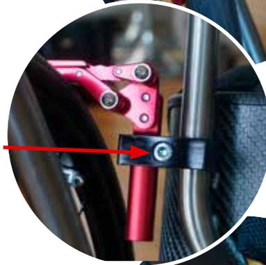
*Loosen the screw on the underside of the bracket.*
