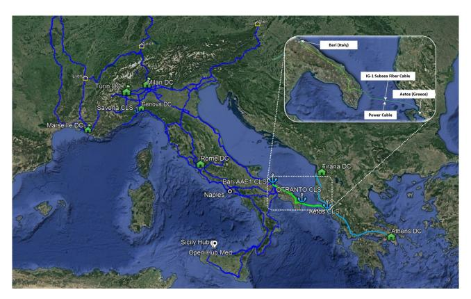
The new upgraded path, as shown between Bari and Aetos in the above graphic, will effectively create an expanded digital highway that bridges Western Europe and the Balkan Peninsula with 400Gb technology, making large volumes of bandwidth available to meet growing demand while also fueling technological innovation in the region.
