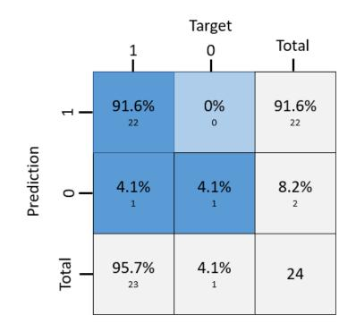
One part over the 24 was not predicted correctly. It was predicted false positive i.e. unacceptable instead of acceptable. Otherwise, the rest of the parts was predicted correctly.
