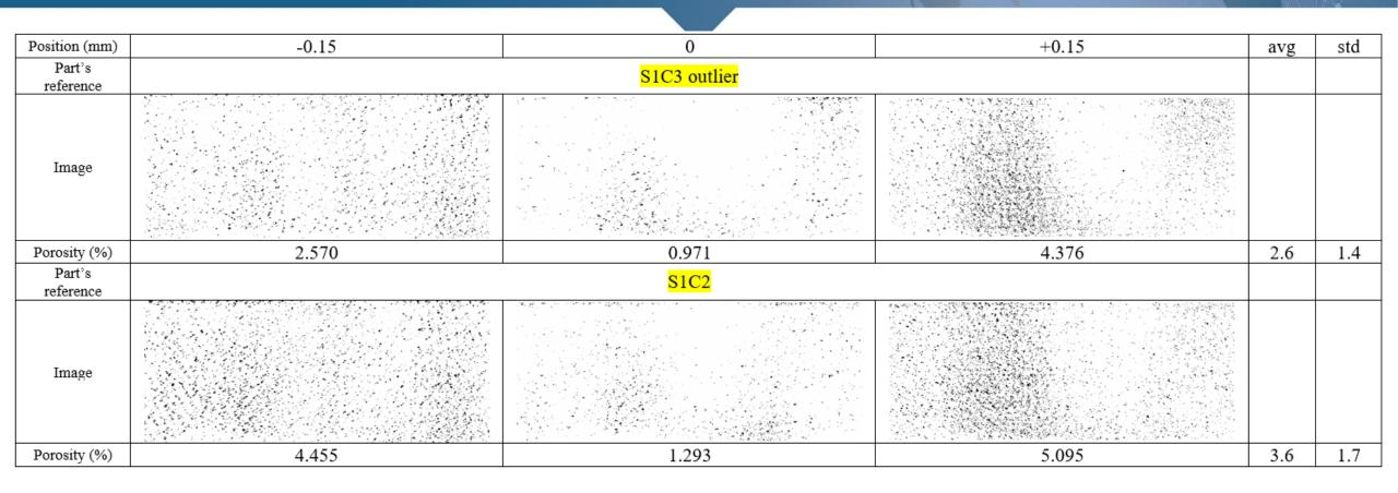
$\Rightarrow$  The differences between the parts, produced with the same parameters, can be assigned to a difference in porosity levels and/or the uneven distribution of the porosity and therefore a difference in overall material modulus.
