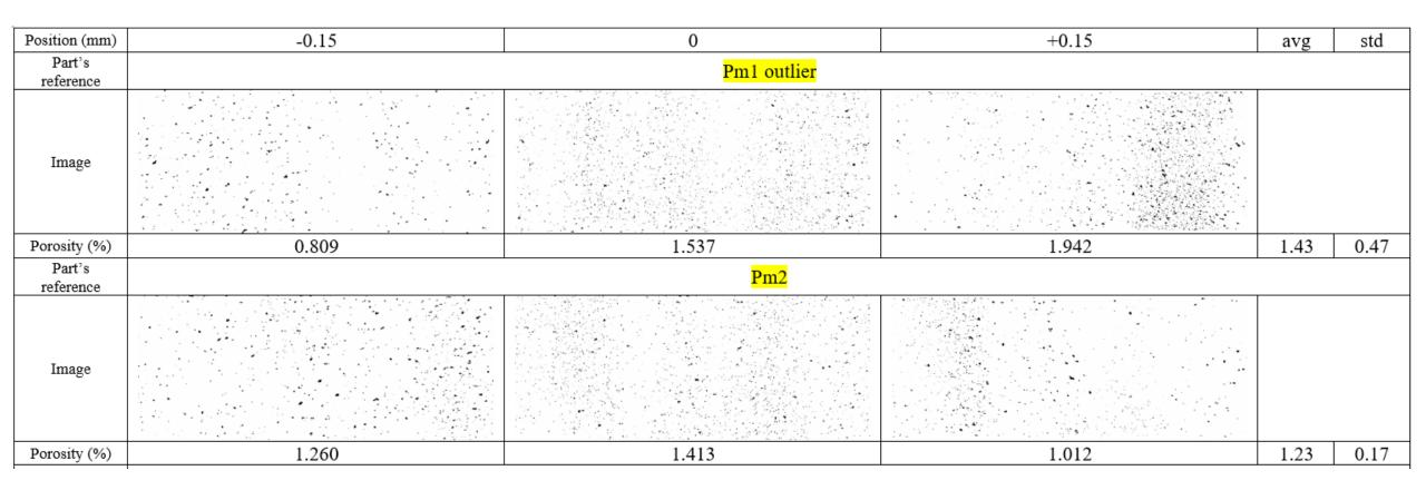
3 different layers on the cylinder element: in the center (defined as position 0 mm) and then on both borders (defined as position -0.15 mm and +0.15 mm from the center)
