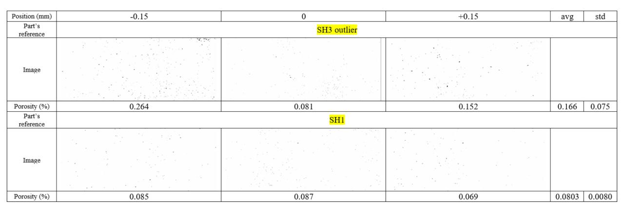
3 different layers on the cylinder element: in the center (defined as position 0 mm) and then on both borders (defined as position -0.15 mm and +0.15 mm from the center)
