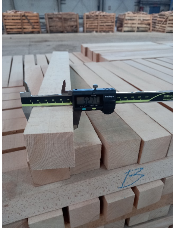
Measurement of moisture content and of dimensions on 50mm x 50mm elements, B grade, premium.
