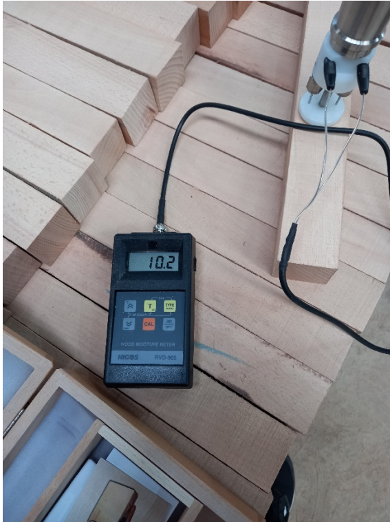
Measurement of moisture content and of dimensions on 50mm x 50mm elements, B grade, premium.
