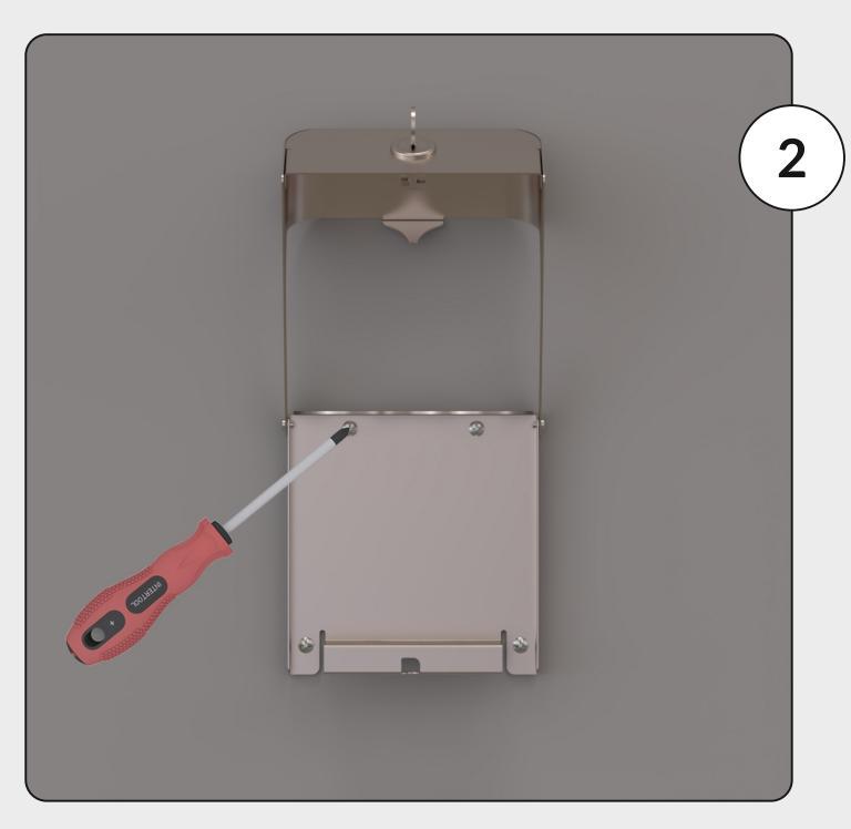
Lift the cover and locate and install the unit with the fixings provided making sure the head is also screwed in to the height of the bottle (The head is adjustable for different bottle sizes).
