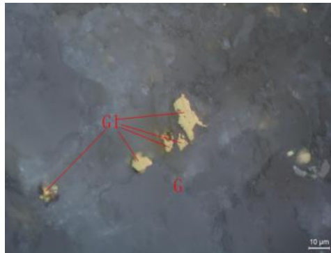
Figure 1. Natural gold (Gl) is distributed in gangue minerals in granular form (Reflection picture of optical microscope)
