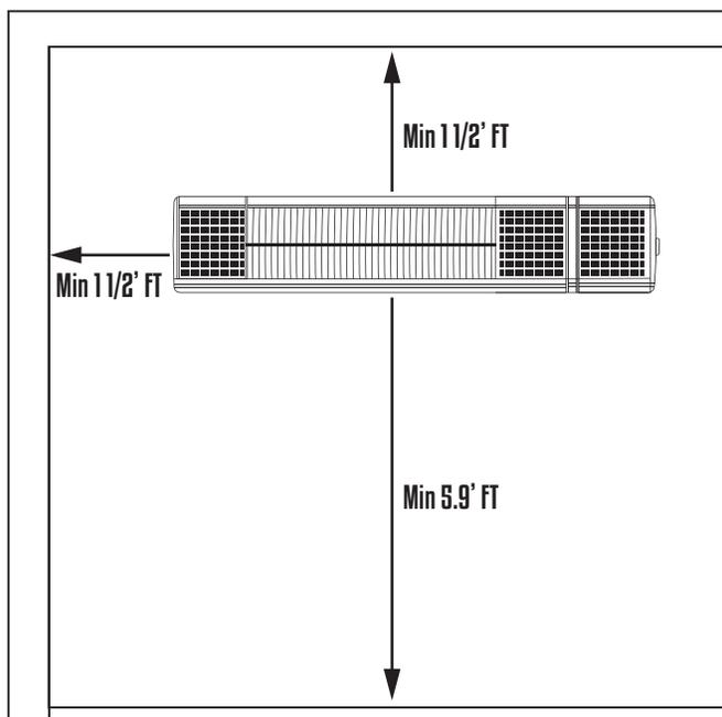
For the safe use of the product, the product installation position should guarantee the bottom minimum height of 5.9 feet from the ground, ceiling, roof, or other coverings minimum distance is 1 1/2 feet, minimum distance with both side walls is 1 1/2 feet (as shown above).
