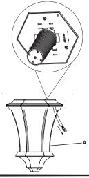
Thread hex nut [J] onto the j-bolt (I). Make sure the hex nut is threaded down the j-bolt far enough for the top of the j-bolt to fit through the mounting plate (II) and the lamp post base (B) with enough threads to secure the base to the j-bolts with acorn nuts (K). Repeaat steps for other i-bolts.
