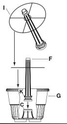
Attach lower post (F) to lamp post base (C) using 3 screws (K) if you have not already done so.
