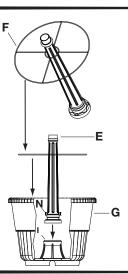
Attach lower post (E) to lamp post base (I) using 3 screw (N) if you have not already done so.
