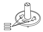
Allow lantern to charge for at least 8 hours in full sunlight with the ON/OFF switch in the OFF position. The ON/OFF switch is located under the solar panel (See Figure 7, page 5). Once the batteries are fully charged, set the ON/OFF switch to ON. If the lantern doesn't turn on after initial charging, ensure batteries are making contact with the terminals.
