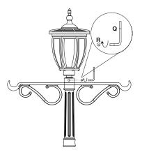
Thread hex nut (H) onto the j-bolt (G). Make sure the hex nut is threaded down the j-bolt far enough for the top of the j-bolt to fit through the mounting plate (N) and the lamp post base (B) with enough threads to secure the base to the j-bolts with acorn nuts [1]. Repeaat steps for other j-bolts.
