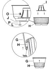
Attach lower post (F) to post base (J) using screws (D) in 3 places. Lower the support ring (G) down the post until it rests on the top of the upper planter (H).
