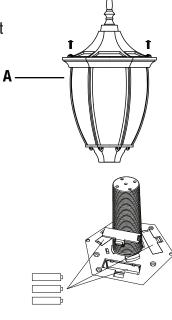
Allow lantern to charge for at least 8 hours in full sunlight with the ON/OFF switch in the OFF position. The ON/OFF switch is located under the solar panel. Once the batteries are fully charged, set the ON/OFF switch to ON. If the lantern doesn't turn on after initial charging, ensure batteries are making contact with the terminals.
