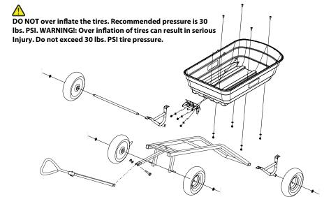
Secure Lock (latch) (D) using push bolts (K) through the tray (A) with slotted head on the inside of the tray (A) as shown in illustration.
