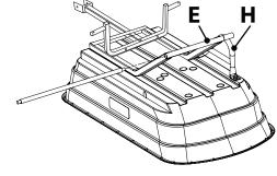
Slide one wheel (G) onto each axle end of the frame (E) with tire stems facing out. Secure with washers (O) and split pins (J). The rear axle (F) may need to be repositioned so that it protrudes through each wheel (G).
