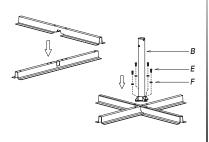
Insert the stem of the Solar Umbrella Assembly (A) into Umbrella Pole (B), turn screw in knob clockwise until tight as shown.
