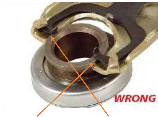
Retaining clip on the outside of bearing
