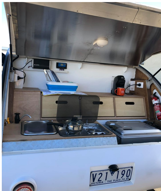
GoPod 90 Kitchen. You can see gas valve on the left hand side of kitchen
