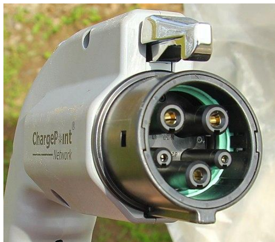
Figure 9: SAE J1772 connector, available around the United States
