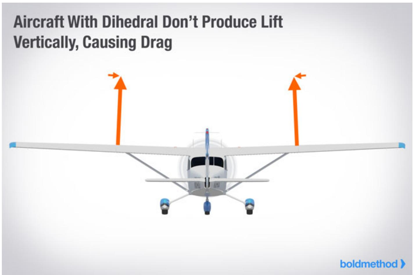
Wings with dihedral don't produce lift completely vertically. There's a vertical component, and a horizontal component. So when you're flying straight and level, your lift is not 100% vertical.
