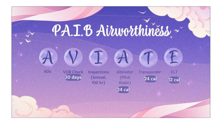
ELT: every 12 cal months. First five minutes of the hour. Replaced or recharged when the transmitter has been in use for more than 1 cumulative hour; or
