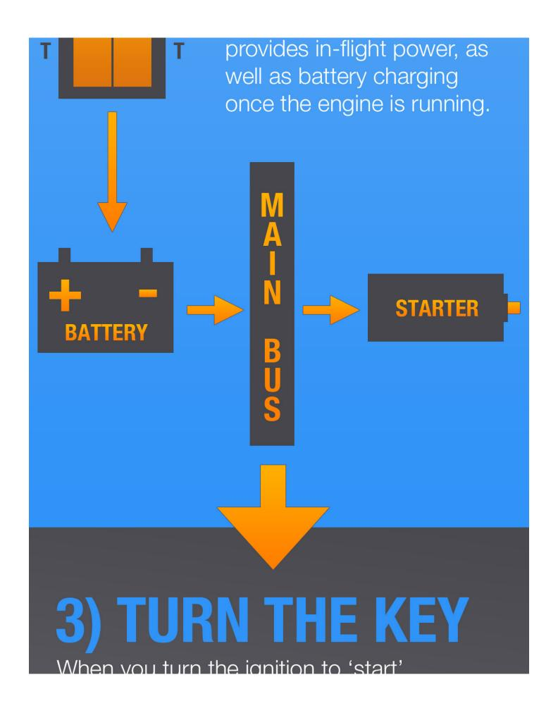
the starter draws electricity from the battery and begins spinning. BOTH • START OFF • **STARTER BATTERY**
