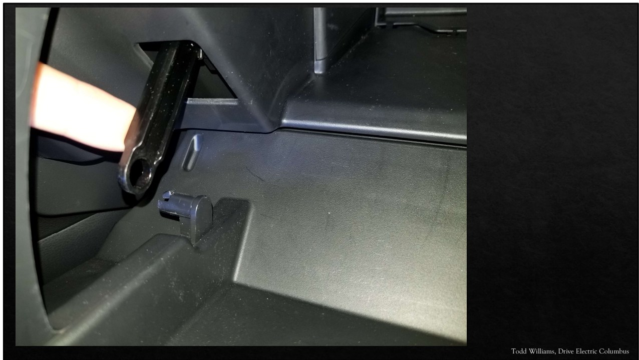
LEAF – Glove Box Hinge Damper – Plastic Spring Clip disconnected
