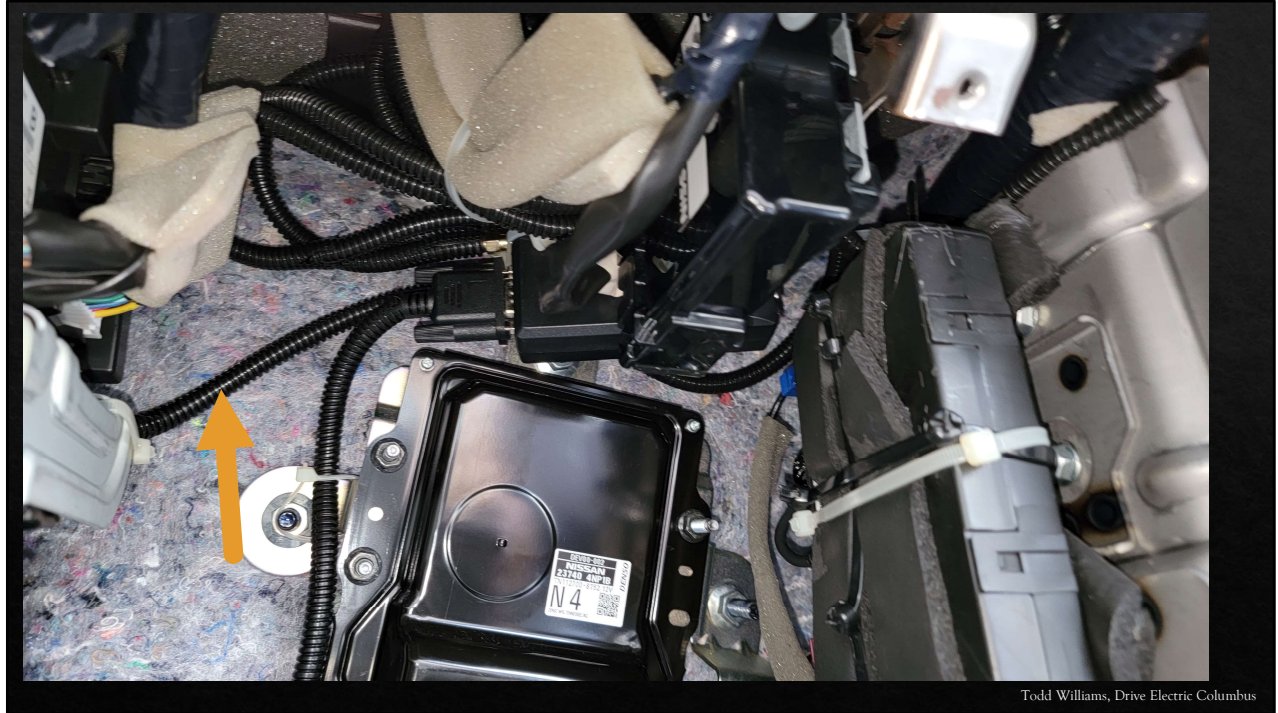
GPS antenna cable in loom routed to be zip-tied up with the other wrapped cables above the ECU module
