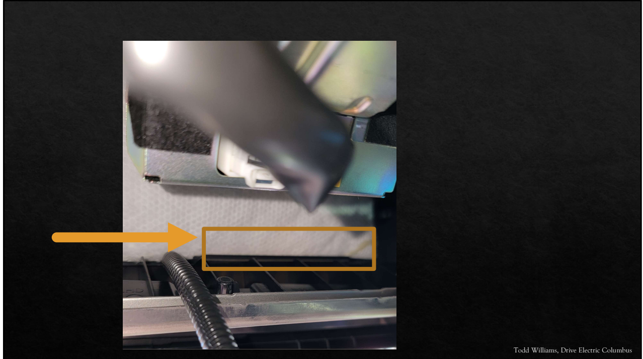
LEAF GSM Cellular Antenna "shelf" location shown from an underside view, looking upward (toward the sky from the bottom of the passenger footwell)
