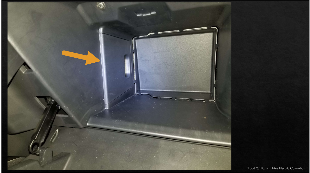
LEAF – Glove Box interior, removable flap cover on left
