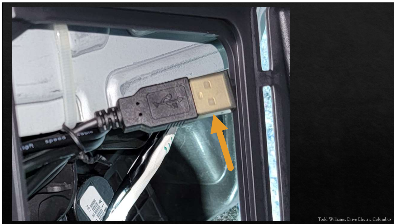
LEAF – Glove box interior with cover removed, USB Micro cable end with USB port cover (optional, sold separately)
