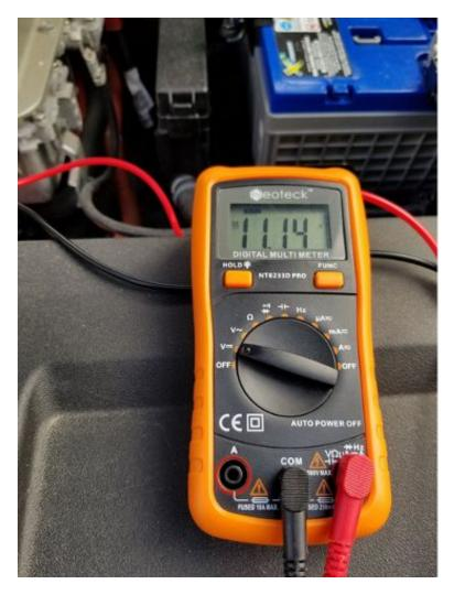
A battery that reads less than 12 Volts is deeply discharged and may end up leaving you stranded somewhere.
