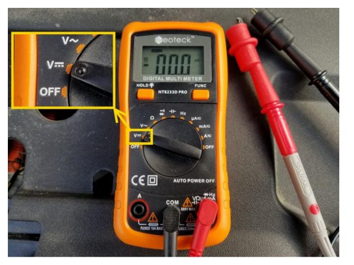
Turn the setting to measure DC voltage, as shown.
