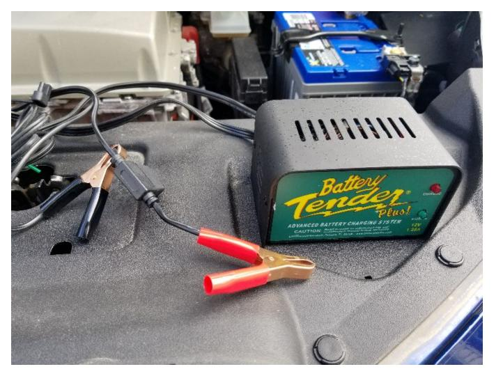
Here is an example of a long-term smart battery maintainer, computer controlled with safety features
