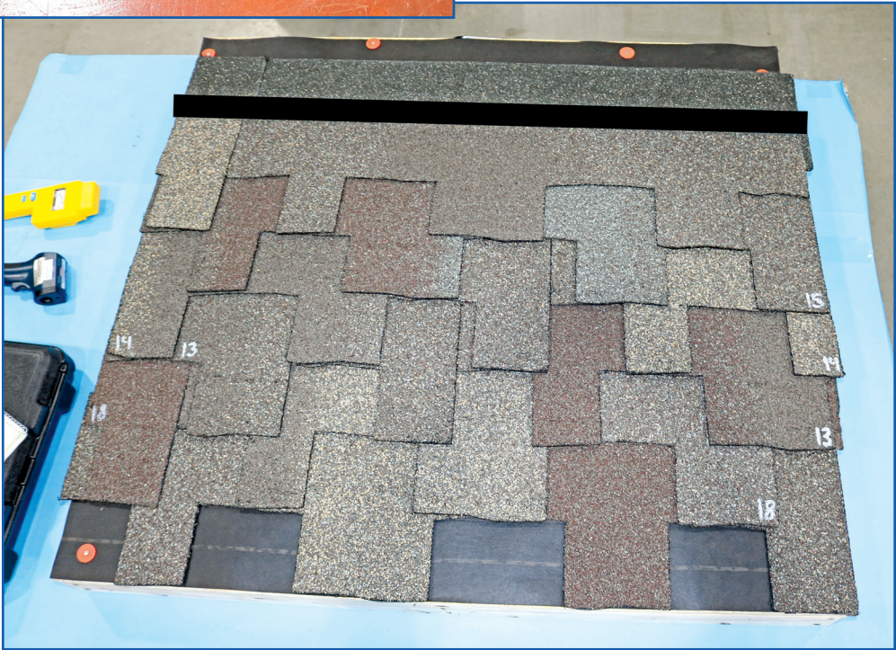
Figure 5 – High-profile shingle test panel.
