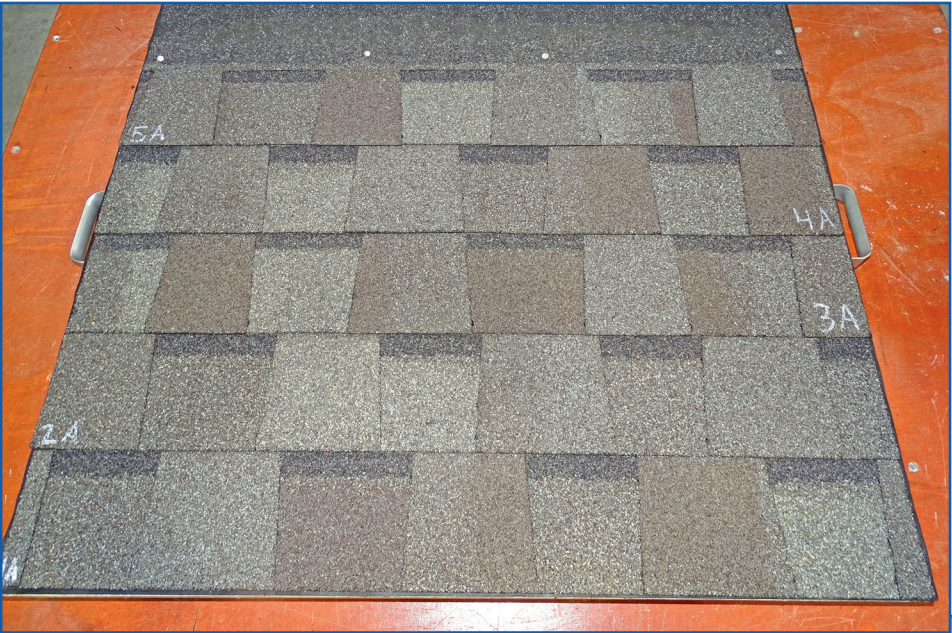
Figure 4 – Laminated shingle test panel.
