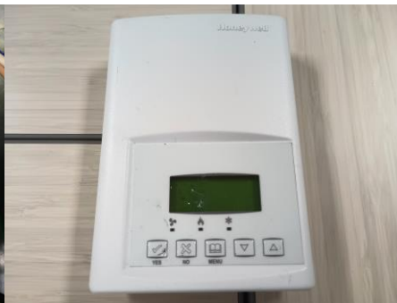
Photo 8 - Honeywell TB7200 BACnet Air-Handling Unit Thermostat
