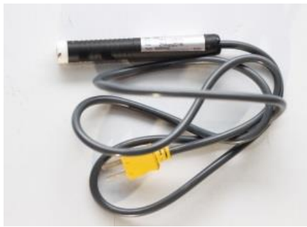
Photo 155 - Surface Probe (Fluke 80PK-3A)
