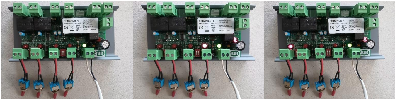
Photo 83 - Normal State (No Device Status LEDs Illuminated)
