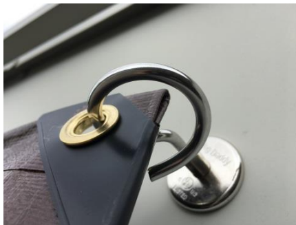
Photo 119 - Magnetic Hangers for Tarp Support
