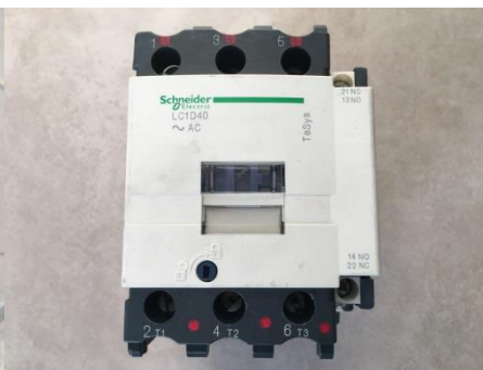
Photo 60 - Enclosed Contactor Design
