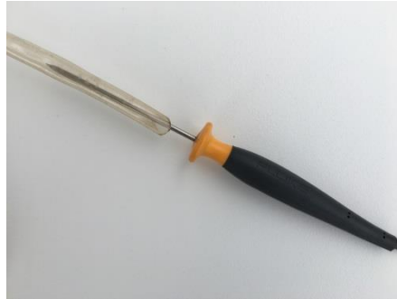
Photo 179 - Temperature Testing of Fluid with Piercing Probe
