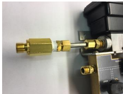
Photo 176 - Attach Hose Adapter to High Pressure Port
