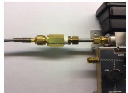
Photo 177 - Calibration Pump Connected to HDPS
