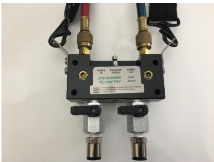
Photo 166 - Hydronic Differential Pressure Module
