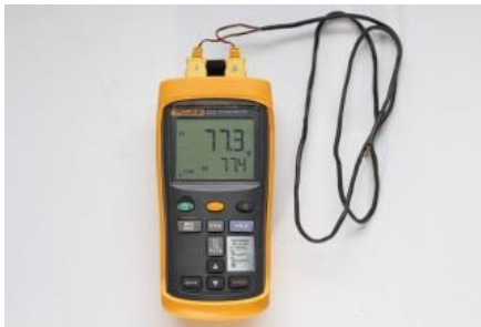
Photo 148 - Thermocouple Thermometer (Fluke 52-II)
