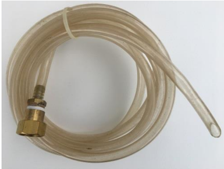
Photo 178 - Test Hose with Hose-End Drain Adapters
