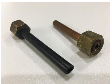
Photo 172 - Compression Fittings for Pneumatic Test Connections
