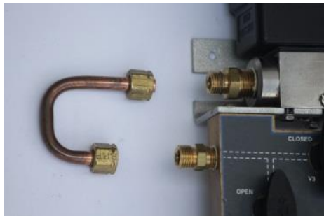
Photo 175 - Remove Piping from High and Low-Pressure Ports
