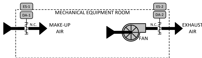
Figure 266 - Exhaust Fan and Supply Air Ducts Controlled with Electric Two-Position Dampers
