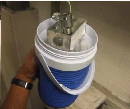
Photo 100 - Immersion Temp. Sensor Placed in an Ice Water Bath
