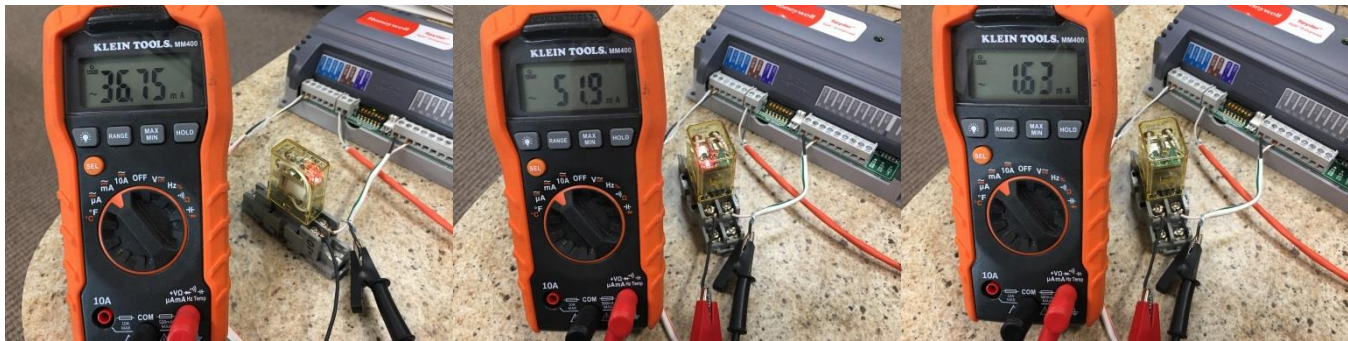
Photo 47 - IDEC RH1B-UL with Binary Triac Output Energized
