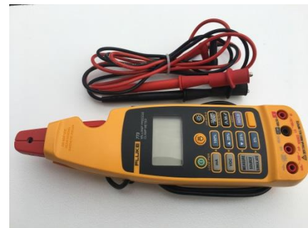
Photo 141 - Process Clamp Meter (Fluke 773)
