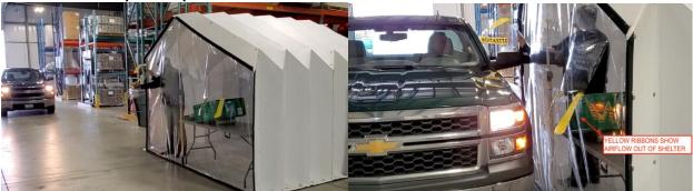
Ontario's EMAT using UniFold shelters in negative pressure bio-containment mode
