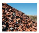
Crushing bricks that are damaged or unsuitable for reuse can be crushed into smaller pieces or fine powder. Crushed bricks can be used as aggregate in road construction, landscaping, or as a base for pathways and patios. Fine brick powder can be used on sports surfaces like baseball diamonds or running tracks. In some cases, crushed bricks can be used as a raw material in the production of new bricks.
