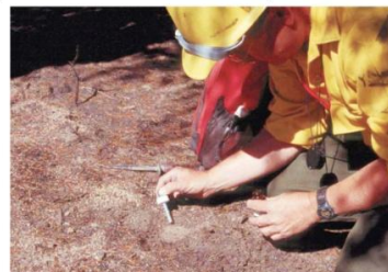
A simple test can determine whether a water repellent layer is present.
