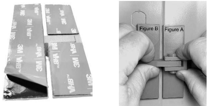
With the alignment pin installed, remove the transfer tape liner from the back of both attachments. Attach Figure A (female receiver) on the fixed panel cover, along the edge adjacent to the circuit breaker access door. Then, attach Figure B to the edge of the circuit breaker access door. Press firmly to secure both attachments.
