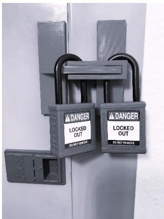
Note: Affix the twin leg receiver to the fixed (non-hinged) surface. Affix the single leg attachment to the face of the hinged cover. The single leg attachment closes between the twin leg trough when the cover is closed and allows for the connection of one, or multiple padlocks.
