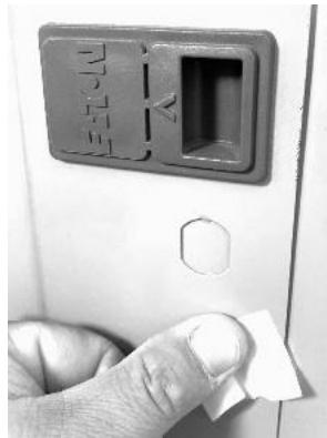
Clean dust and oils from mounting surfaces using an isopropyl alcohol wipe.
