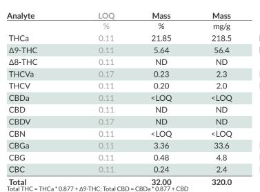
$LOQ = Limit \ of \ Quantitation, \ ND = Not \ Detected; \ Unless \ otherwise \ stated \ all \ quality \ control \ samples \ performed \ within \ specifications \ established \ by \ the \ Laboratory.$
