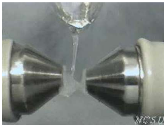
Photograph showing liquid oxygen being trapped in a magnetic field due to its paramagnetic nature.
