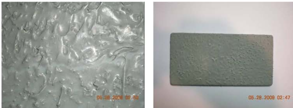
Figure 2. (Left Photo) Surface of MC-156 coated panel following 3500 hours in 5% salt solution. (Right Photo) MC-156 coated Luminore panel following 5000 exposure to 5% salt solution.
