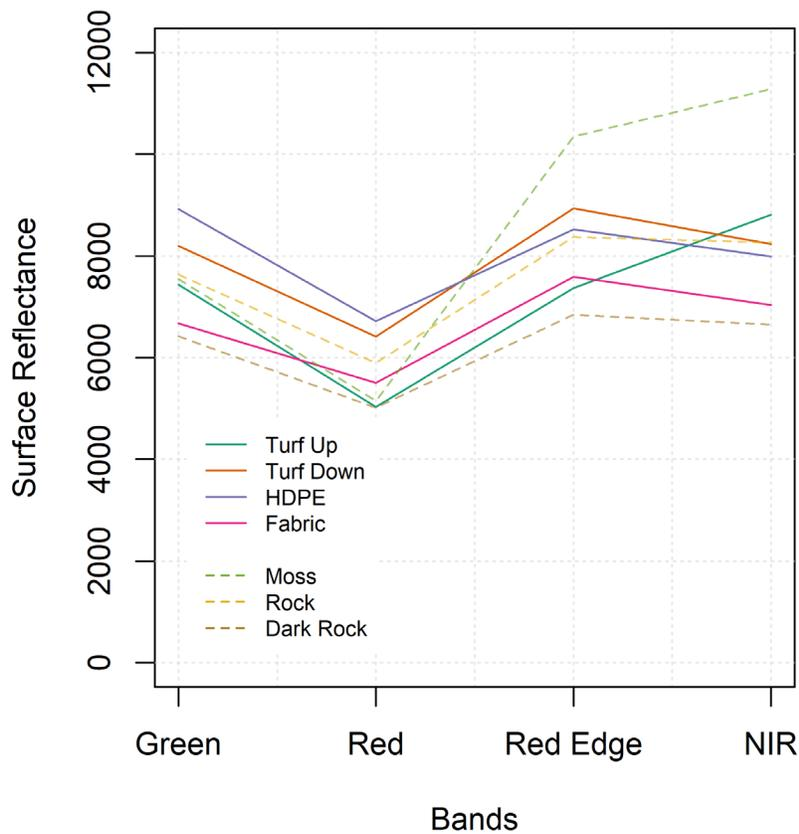
**Figure 2** Graph illustrating average spectral band overlap between debris types and natural terrain.
