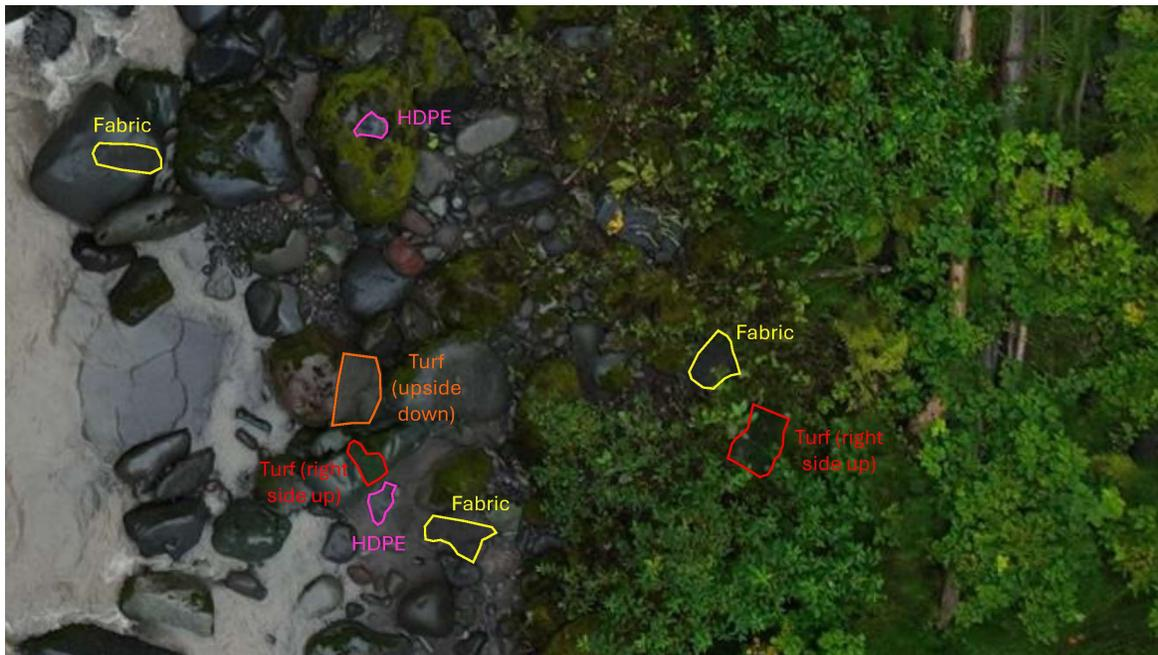
**Figure 1 Sample debris placed along river for multispectral camera calibration.**
