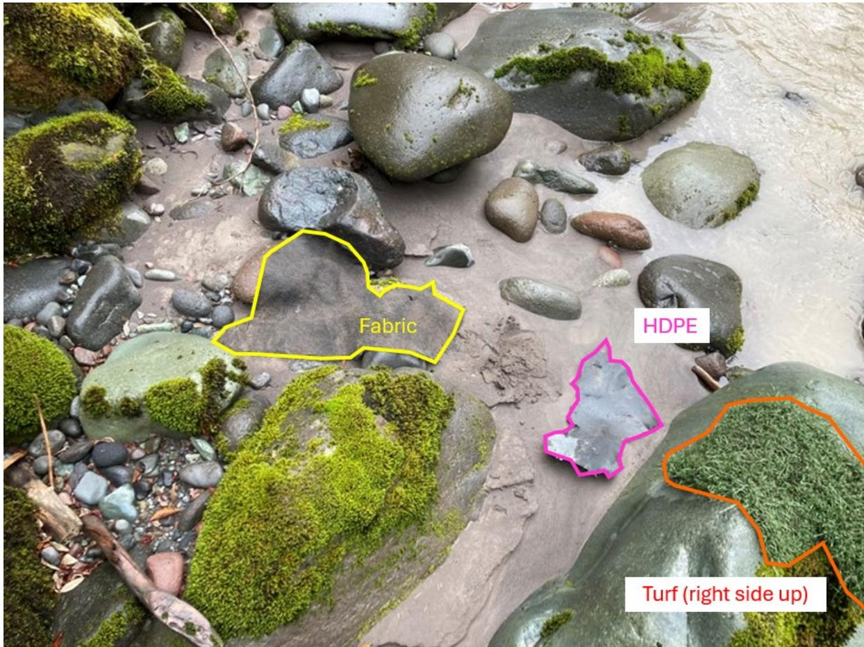
**Photo 2** Sample debris placed on river right for camera calibration flight. From right to left: HDPE, fabric, and right side up turf.
